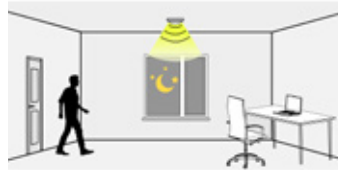
Presence detected, insufficient daylight, all lights on
