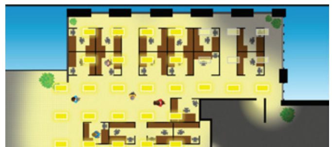
4. As more workers enter, the lights dim up accordingly.
