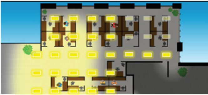
7. As people begin finishing work, additional lights dim down.
