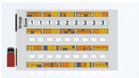
1. Luminaires can be grouped together or further divided into zones
