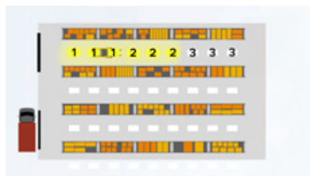
2. Luminaires in top aisle dim up to task level by zones when motion is detected
